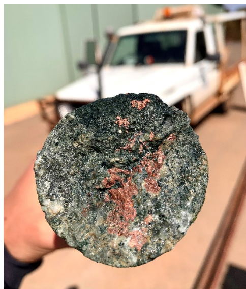
Figure 9 LEFD007a Native copper in fracture plane drill core 152.53m
