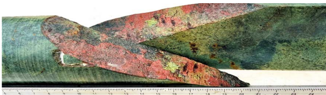
Figure 4 LEFD006 interval 224.5 to 224.8m shows high-magnesium Western Basalt, mineralised by native copper along fracture plane with a gypsum film, with epidote alteration and minor ex-sulphides (LEX ASX release 1 August 2022)
