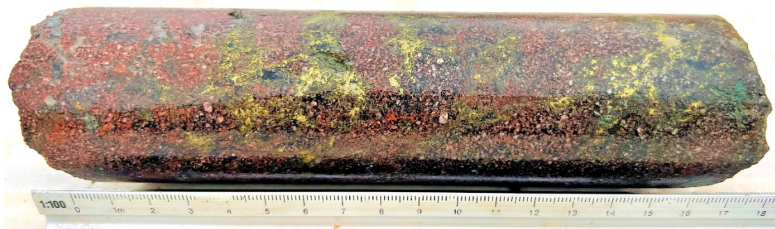
Figure 5 LEFD006 interval 435.6-435.8m showing Burns diorite porphyry altered by pervasive hematite, cross-cut by chalcopyrite and pyrite stringer veining (LEX ASX release 1 August 2022).
