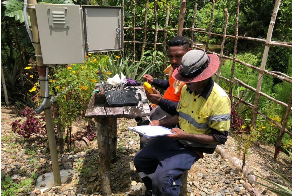
Figure: Misima team extracting data from the Hydroquest iRIS 150FX data logger at Kubwal
