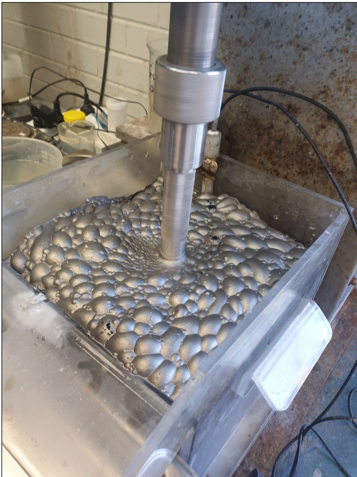
Figure 2: Flotation of Nickel Sulphides from C2 Deposit
