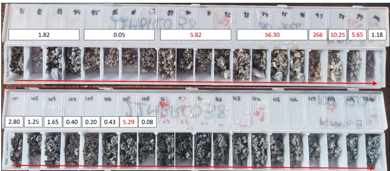
FIGURE 1: RC CHIP TRAYS 80 TO 120M DOWNHOLE IN 22MBRC038 WITH HIGHLIGHTED ASSAY VALUES. ARROWS SHOW THE DOWN-HOLE DIRECTION. WRITTEN NUMBERS ABOVE EACH SEGMENT ARE THE “SAMPLE TO” DEPTH.
