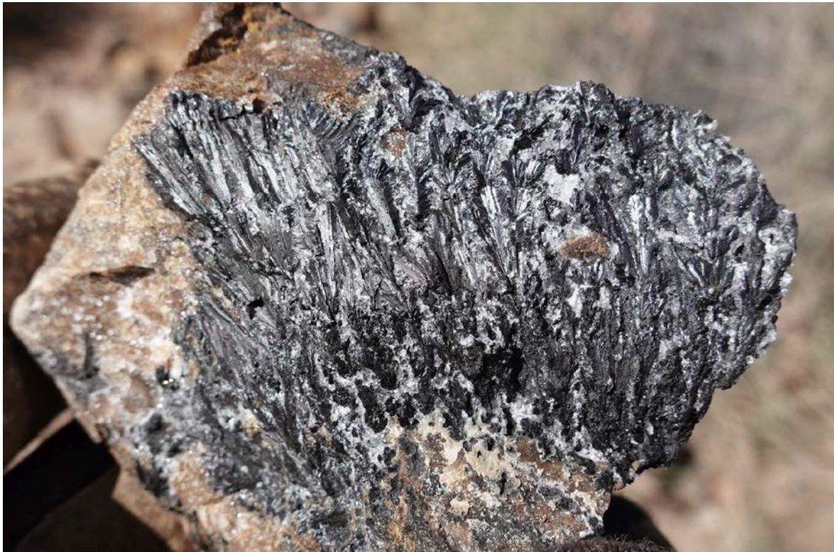
Figure 11. Outcrop of plumose manganese oxides in a jasperoid breccia at Jimmy Creek
