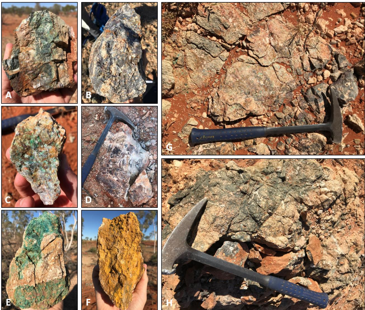
Figure 5 Selection of Ningaloo rock chips including: A) JE0094 with 0.36g/t Au + 1.42% Cu + 957ppm Bi; B) JE0105 with 0.19% Cu; C) JE0098 with 1.27% Cu; D) JE0103 with 0.46% Cu; E) JE0107 with 9.65% Cu + 2.93g/t Ag; F) JE0108 with 0.16% Cu; G) JE0096 with 1.28% Cu; and H) JE0110 with 0.19% Cu. PLEASE NOTE: This photo collage of samples first appears in ASX announcement dated 3 June 2021. The associated assay tables which included sample locations also appears in this previous ASX announcement.
