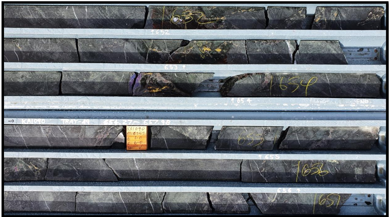
KAI090 – 651.5m – 657.0m interval of bornite-chalcopyrite-magnetite-actinolite-calcite breccia of potassic altered volcanics at Kaiser
