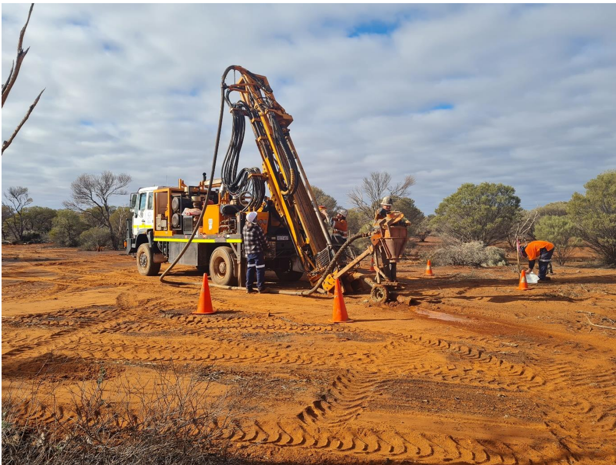
Figure 1, Aircore rig onsite at Kookynie Gold Project
