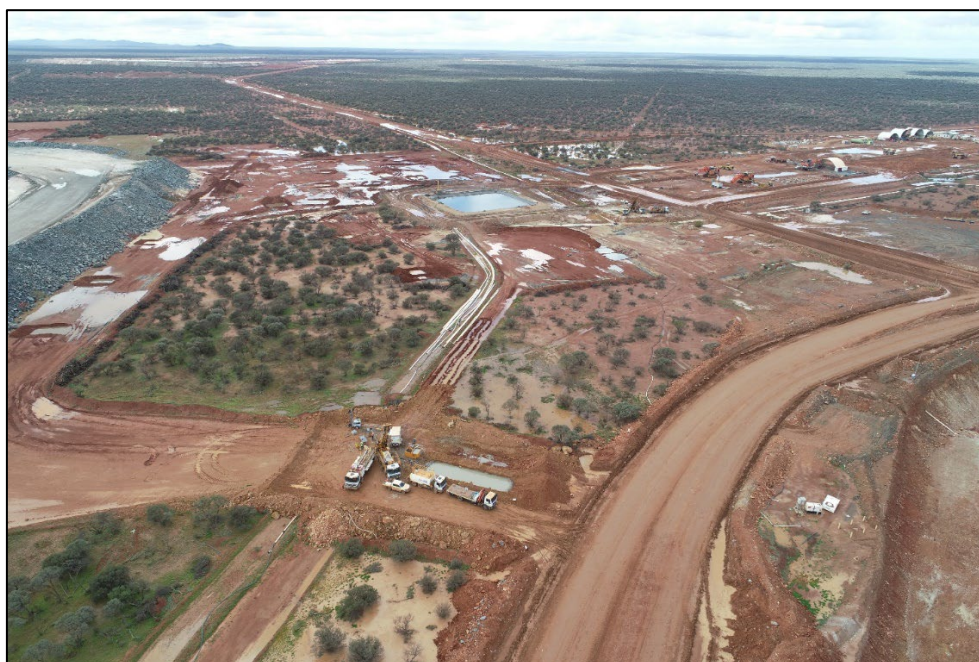
Figure 1: Aerial image of active drilling of the Gilbey’s North - Never Never Gold Deposit during a recent rainfall event. Note: Diamond drill rig in the foreground and RC drill rig to the right of the square “turkey nest” water dam.
