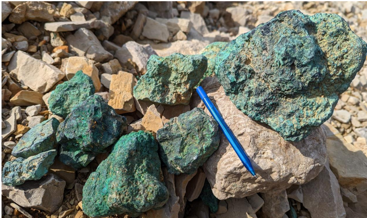
Figure 5: Massive chalcocite boulders exposed at surface from the 2750N Zone.
