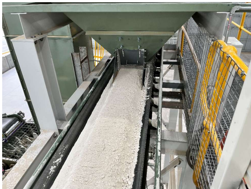
Figure 2. Conditioned ore feed to the rotary kiln
