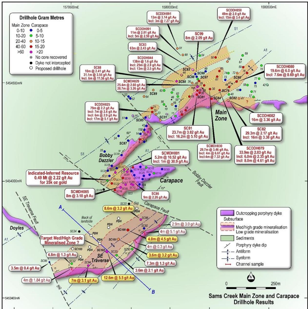
Figure 8. Plan view from SE Traverse - Main Zone showing anticline and drill hole results with mineralised shoots shown in orange.
