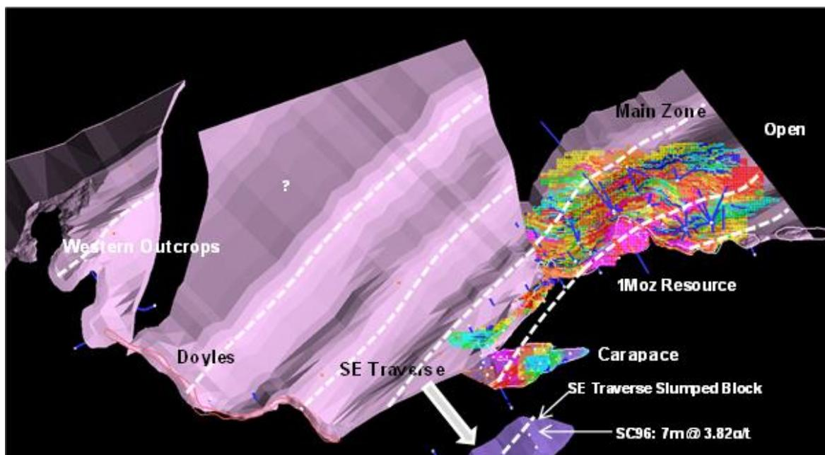
**Figure 5. SCD plan view with mapped and interpreted anticline hinges shown by white dotted lines. High grade mineralisation indicated by magenta and red blocks in the MRE.**
