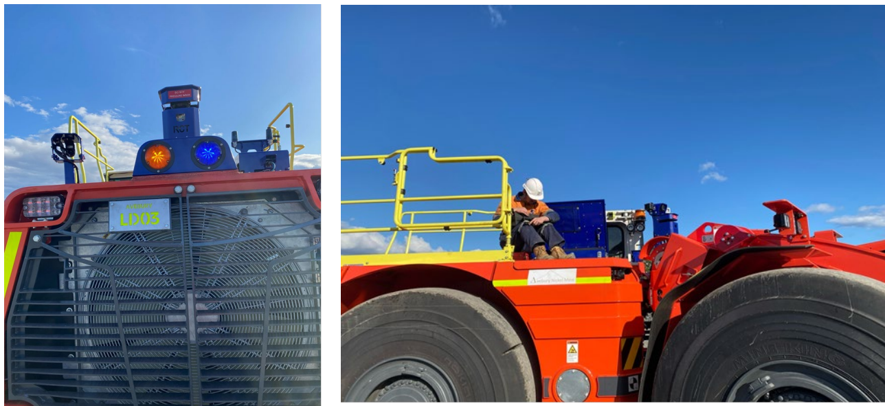
Figure 3. Sandvik loader equipped with remote guidance equipment
