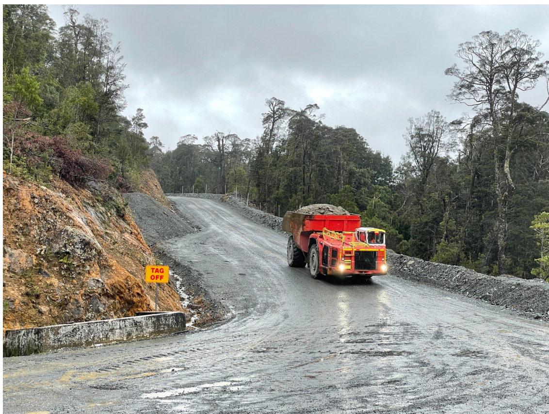
Figure 5. Backloading waste from surface
