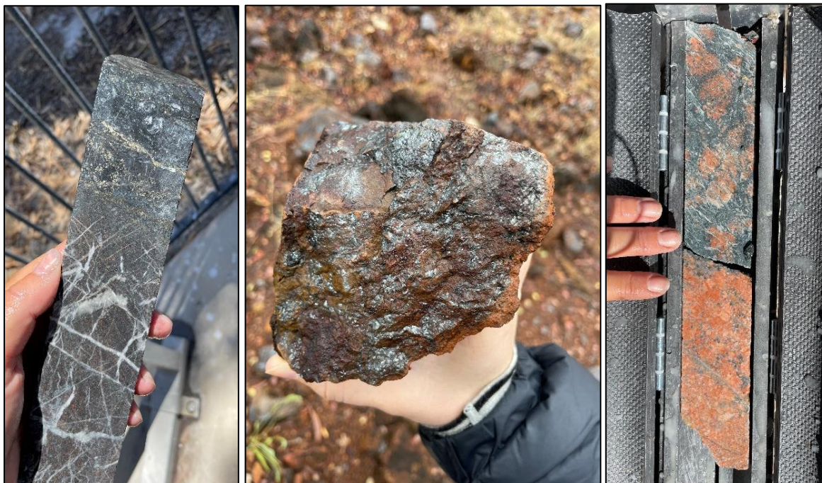
Figure 5 – (From left) Sulphides in altered granite and skarn, specular hematite from a surface outcrop adjacent to GN22_01, and 'red-rock' style alteration in granite
