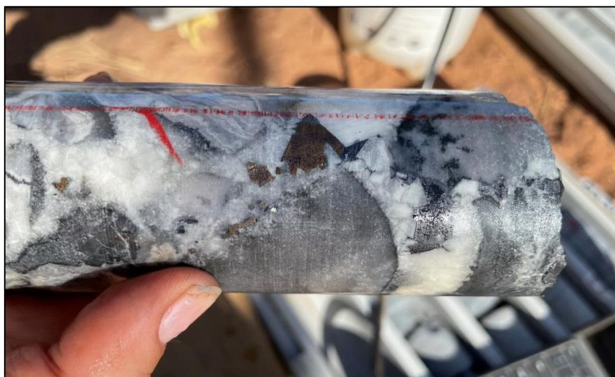
Figure 7 – ‘Slugs’ of silvery galena and angular brown-buff coloured sphalerite filling cavities in a limestone pseudo-breccia (JB22_02).
