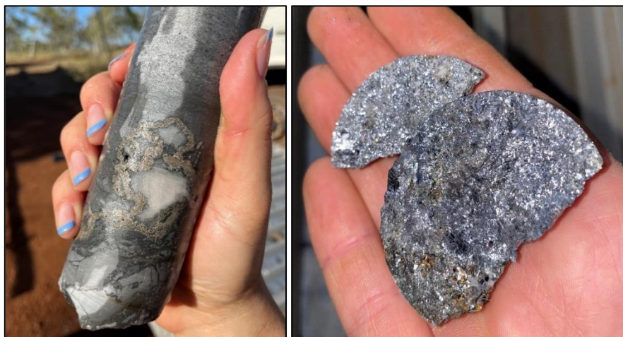
Figure 6 – (left) Buff-coloured colloform sphalerite replacing carbonates in pseudo-breccia (JB22_02) and (right) near-complete replacement of carbonates by galena (with minor sphalerite) in JB22_02.
