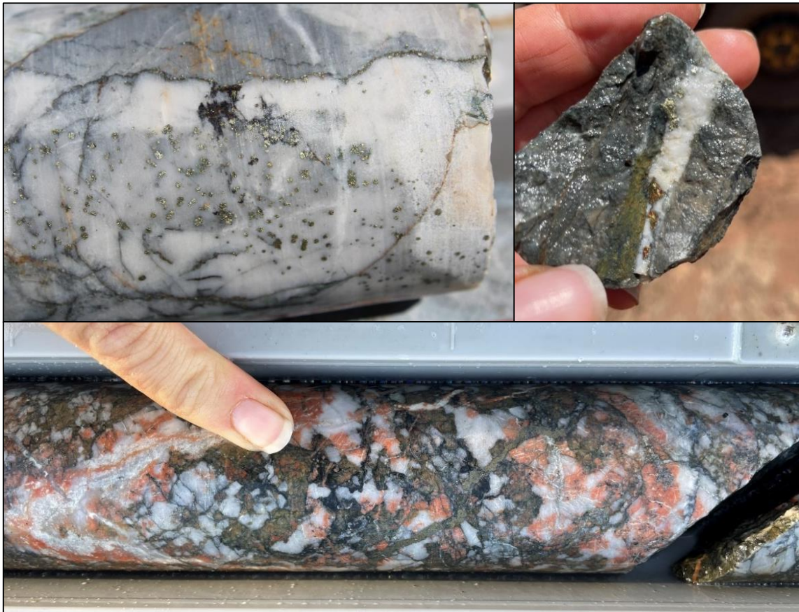
Figure 4 – Clockwise from top left: Remobilised sulphides in wall-rock, associated with seams and veinlets; pyrite and bornite in a quartz vein; brecciation and patchy 'red-rock' style alteration with disseminated pyrite in granite (GN22_02)
