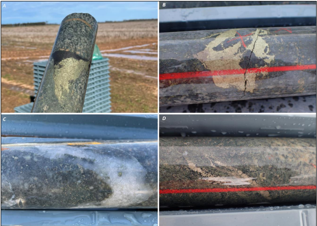
Figure 3. Images of various down hole intervals of HQ drill core (63.5mm diameter) with assays pending from the lower portions of hole 22MYDD415. A) strongly altered diorite with a very large bleb (to ~80mm) of chalcopyrite (yellow) and magnetite (black) from 714m; B) brecciated, chlorite-altered diorite strongly infilled with chalcopyrite and lesser pyrrhotite (brass-coloured) from 730.5m; C) chlorite-altered diorite with abundant disseminated pyrite, cut by quartz-carbonate veins with minor chalcopyrite from 810.2m; D) chlorite-altered diorite with intensely-developed pyrite and trace chalcopyrite from 962m.
