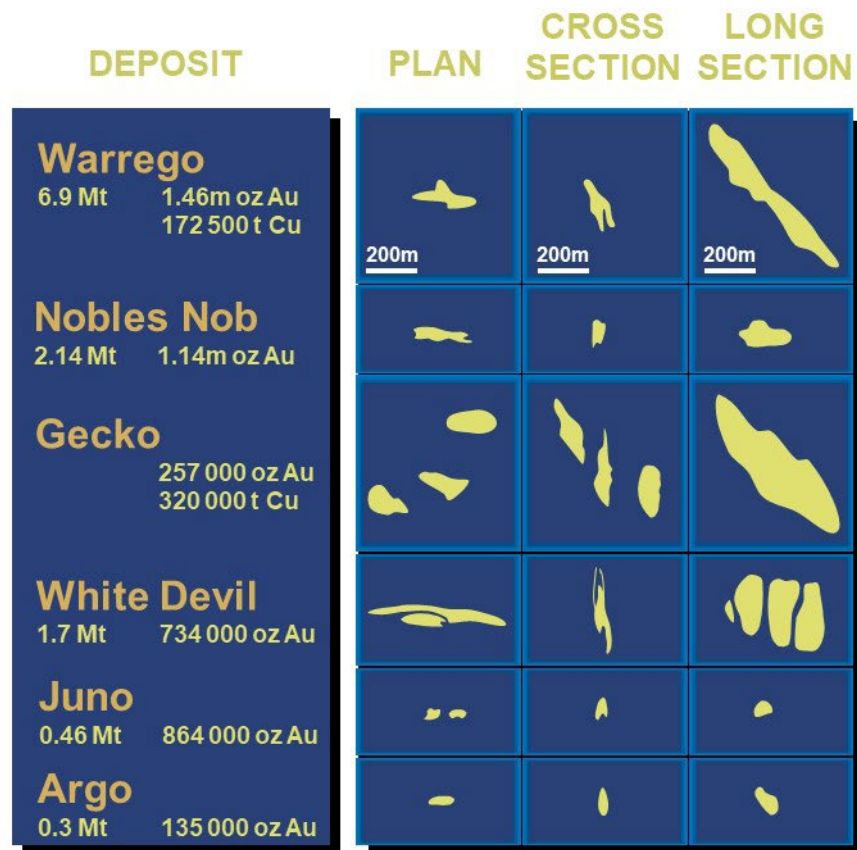
Figure 4: Geometries of Major Tennant Creek Orebodies, noting the typical constrained plan/horizontal footprint.
