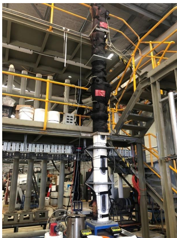
Image 9 | Nifty 6m high metallurgical test work column
