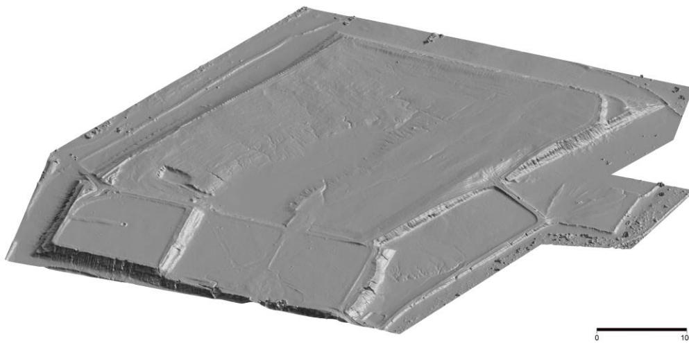
Figure 2: Topographic surface of the Peko tailings generated using the LiDAR data
