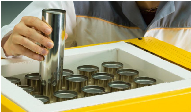
Figure 1 – SAS cells in battery module
