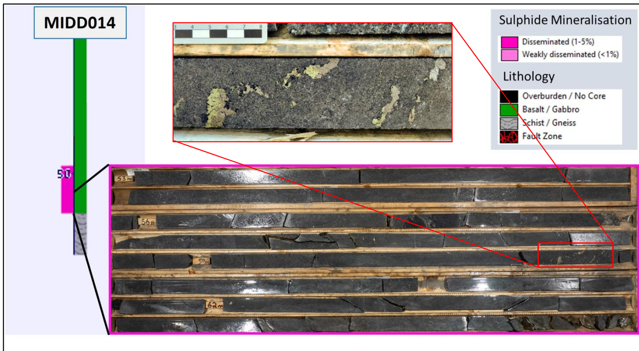
Figure 2: Sulphide mineralisation in drill hole MIDD014 (highlighted in purple). See Appendices 1 & 2 for a summary geological log and the sulphide logging guide.
