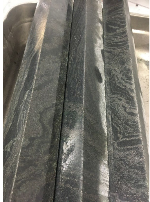
Figure 3. Concentrated matrix magnetite mineralisation.
