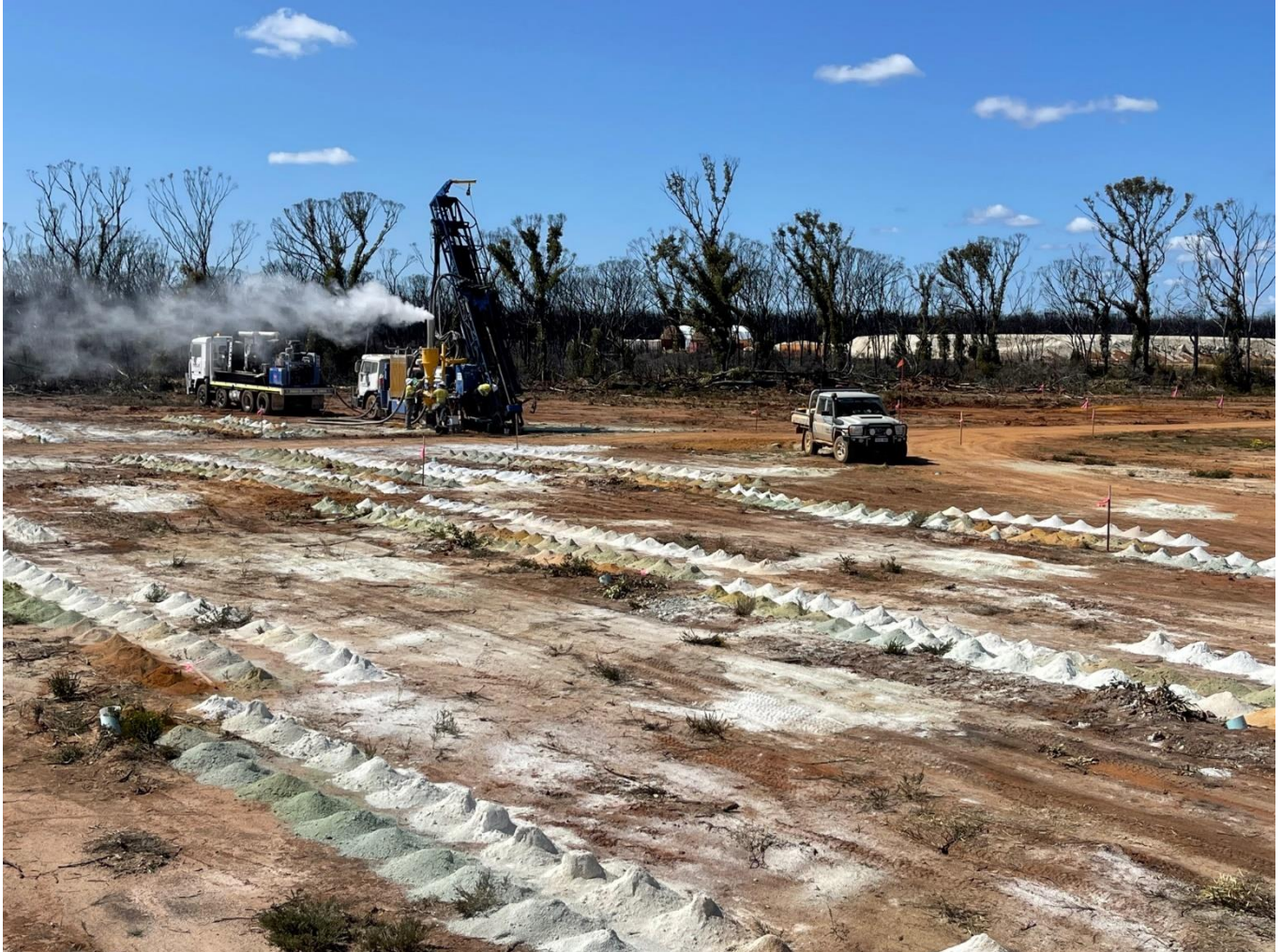
Figure 3: Drill Samples from Infill RC holes at Kat Gap
