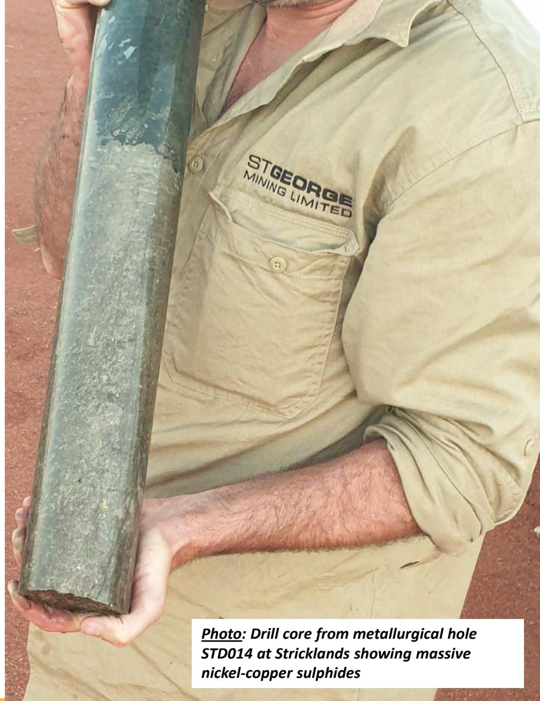
***Photo: Drill core from metallurgical hole STD014 at Stricklands showing massive nickel-copper sulphides***
