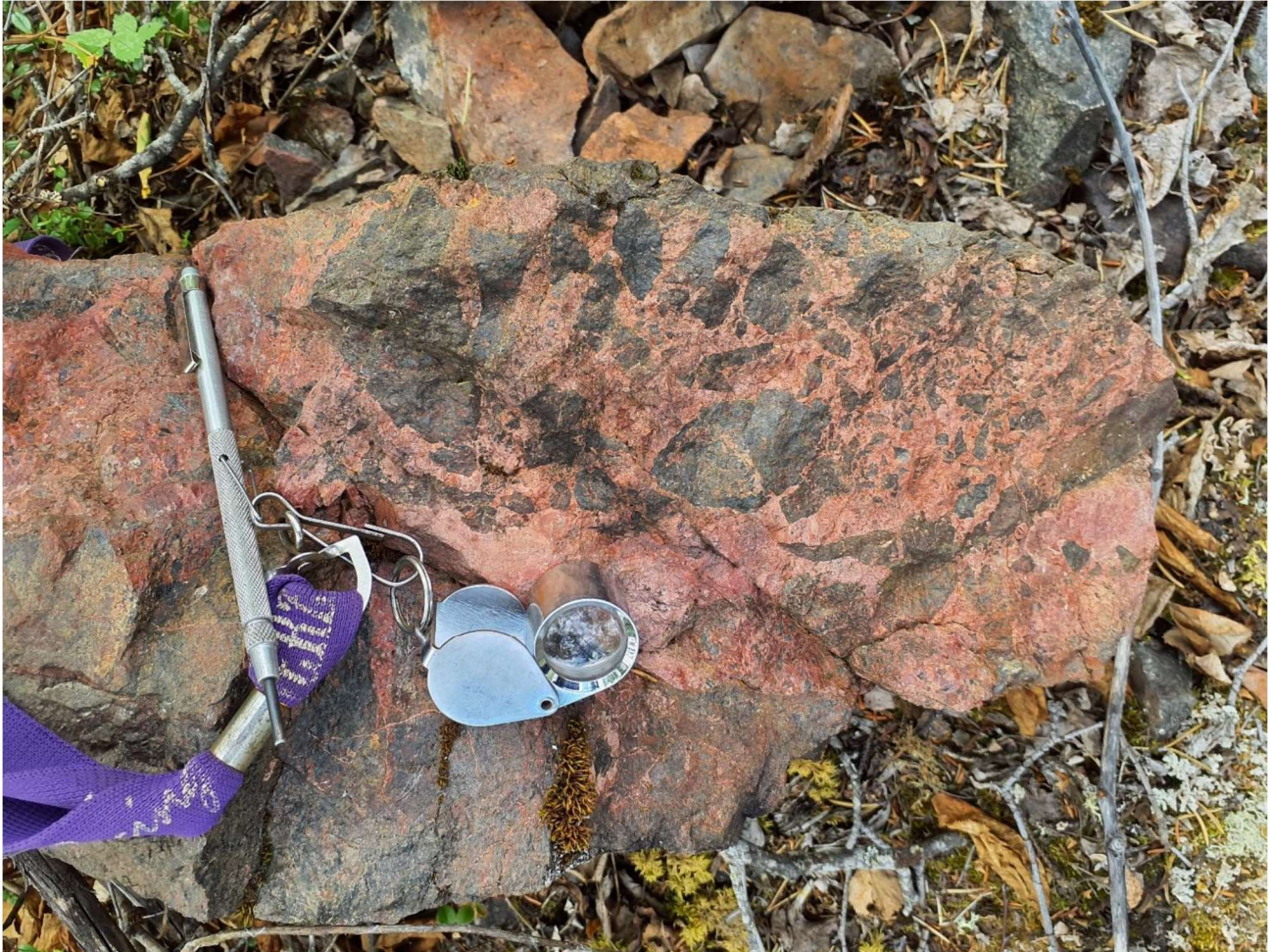
Figure 8: Surprise Creek Fault - Hematitic breccia with U, Cu and Pb mineralisation (max scintillometer reading of 65,535 cps)
