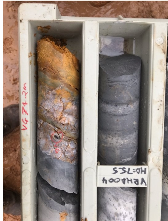
Figure 2 Visible Gold shown in the red circle in the HQ core
