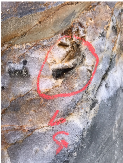
Figure 3 Further Visible gold within the quartz vug
