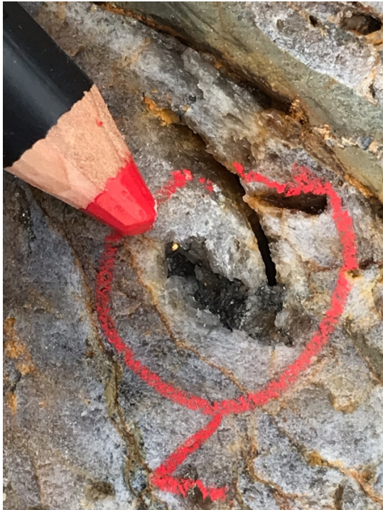
Figure 1 Visible gold in quartz vug
