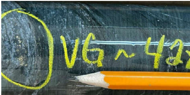
Esker Prospect: 148.0 g/t Au (gold) and 57.0 g/t Ag (silver) from 70.29-70.59m in WP-22-03. 42 specks of visible gold.
