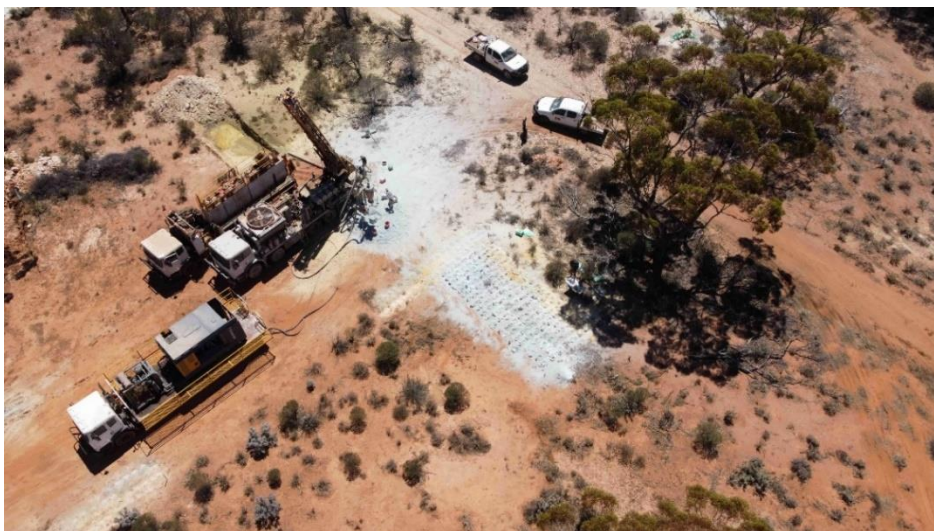
Figure 13. KTE Mining Services RC rig drilling at the Rocky Dam Project.
