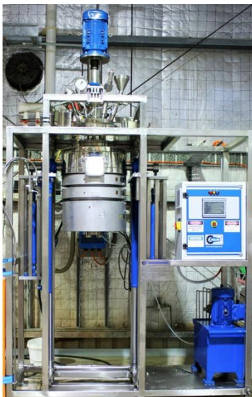
Purpose-built autoclave for LieNA®
