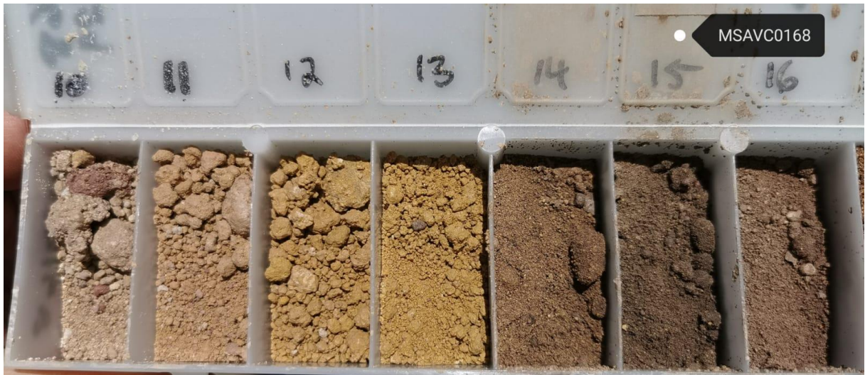
Photo 1: Yttria Rare Earths elements and critical minerals MSAVC0168 with 7m @ 958ppm TREYO + 54ppm Sc 2 O 3 from 9m; inc 3m @ 1693ppm TREYO + 73ppm Sc 2 O 3 from 10m; and 1m @ 2328ppm TREYO from 12m
