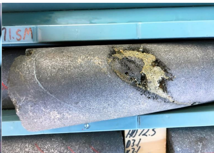
Figure 2b: Massive sulphide bleb with chalcopyrite
