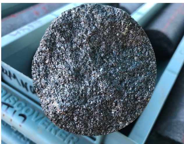
Figure 2a: MND003 vanadium-titanium-magnetite
