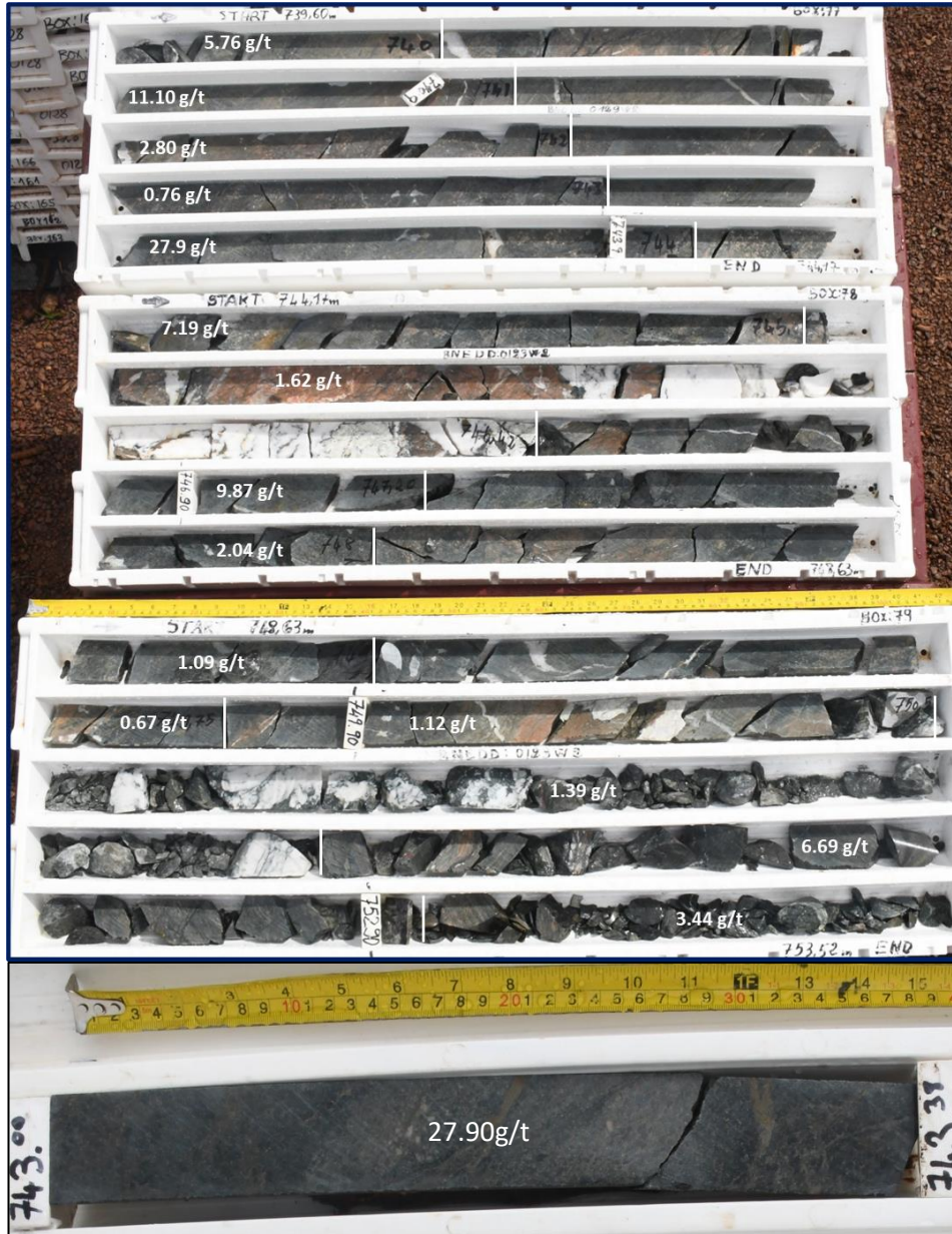
Figure 5 - Section 1174820N BNEDD129W2 Cut core high-grade specimens - +4% Py +/- Cpy + Chlorite + Albite + Silica +/- Feldspar +/- Biotite.
