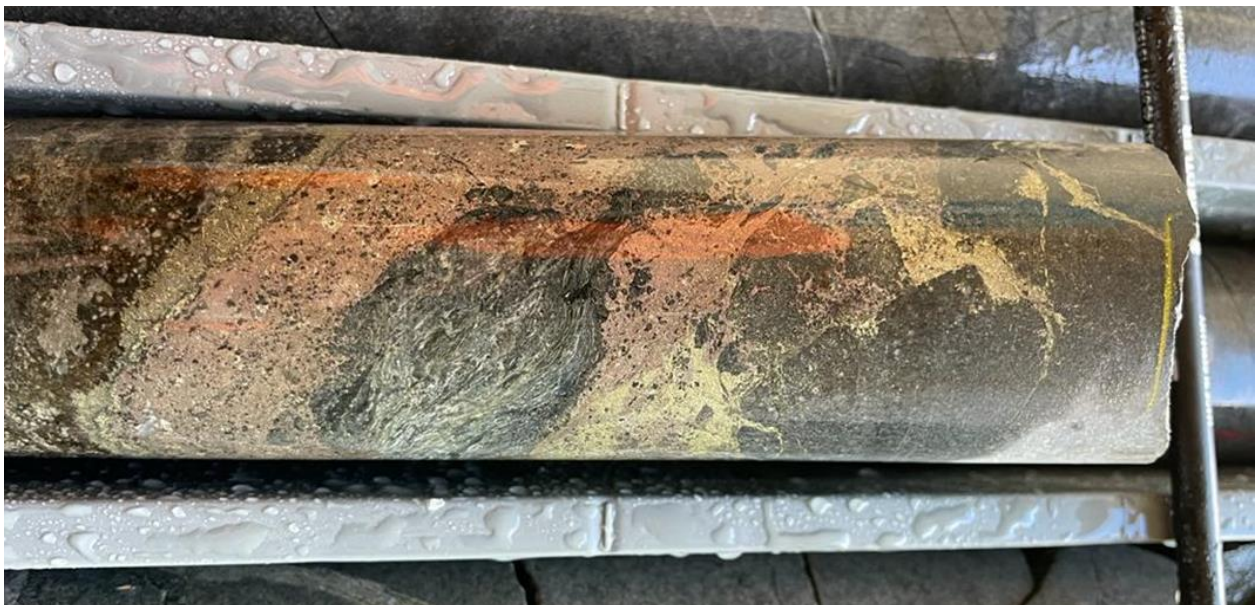
Figure 1: 22B2DD003 (26.8 -27.0 metre interval – NQ core 47.6mm diameter). Strongly mineralised dolerite with fine-grained pyrrhotite, chalcopyrite and coarse minerals of pentlandite. Mineralisation is semi-massive and interstitial. Within a 29.35 metre zone of sulphide mineralisation. 1
