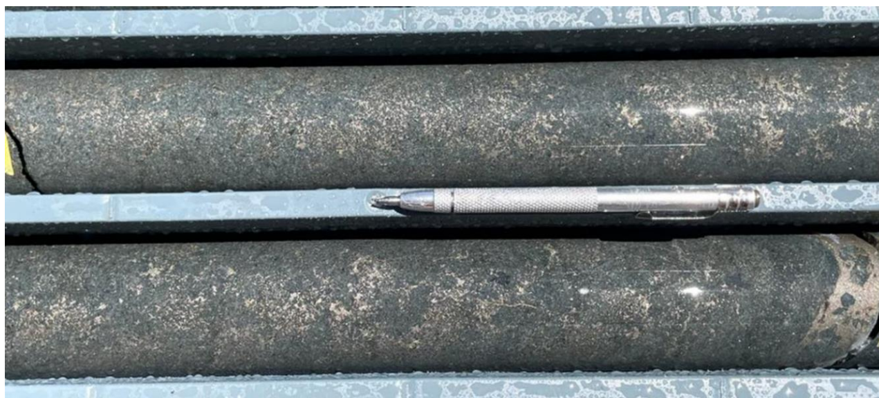
Figure 4: 22B2DD003 (40-42 metres – NQ core 47.6mm diameter) Strongly mineralised dolerite with disseminated angular blebs of fine-grained pyrrhotite and pentlandite with minor chalcopyrite, within a 29.35 metre zone of sulphide mineralisation. 1
