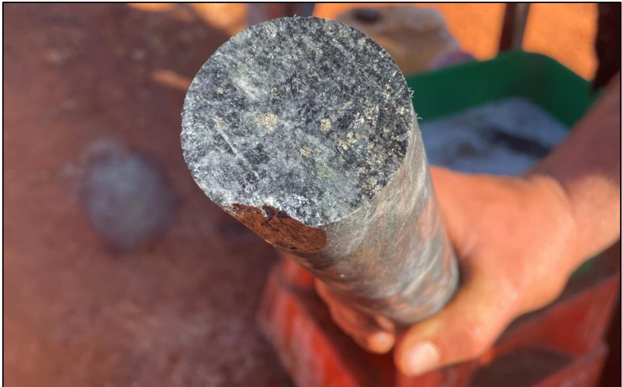
Figure 3: Section of core from drill hole IRN001 displaying disseminated sulphides at the Ironstone Gold Project
