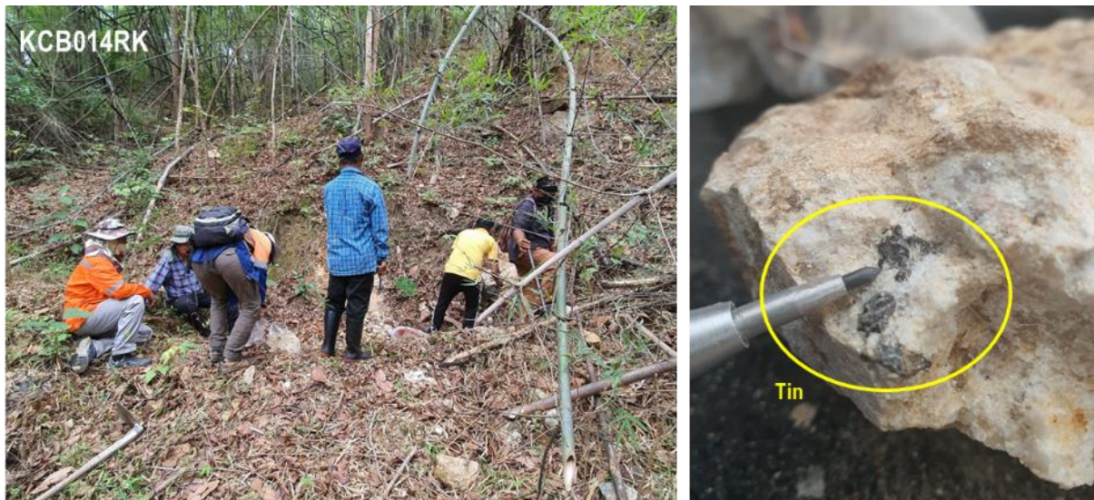
Figure 18: Kanchanaburi sample KCB014RK from outcropping pegmatite showing tin mineralisation. This pegmatite has been mapped over 2km strike, 600m wide and striking NW
