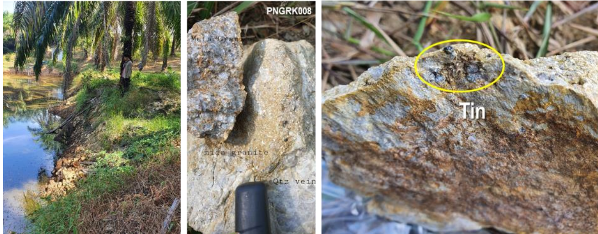
Figure 17: Phang Nga sample PNGRK008 from a water course cutting showing tin mineralisation
