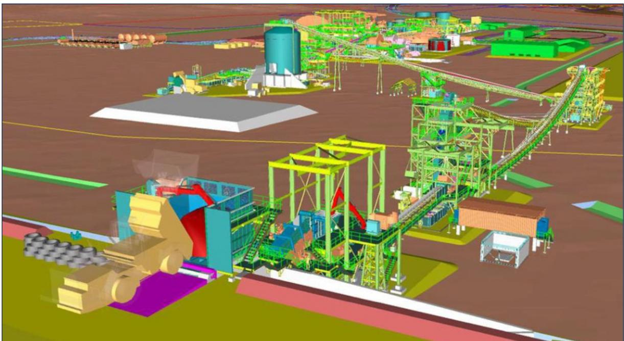
Figure 5: Revised secondary crushing and screening area incorporating lower steel heights and sacrificial conveyor on primary crushing area
