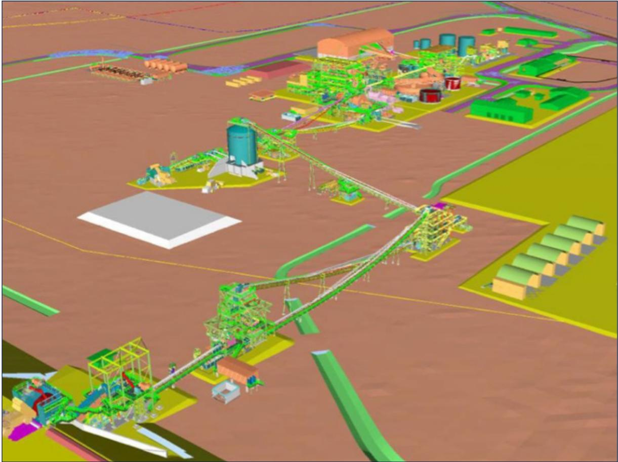
Figure 4: Revised Process Plant layout incorporating closed circuit crushing and large fine ore bin
