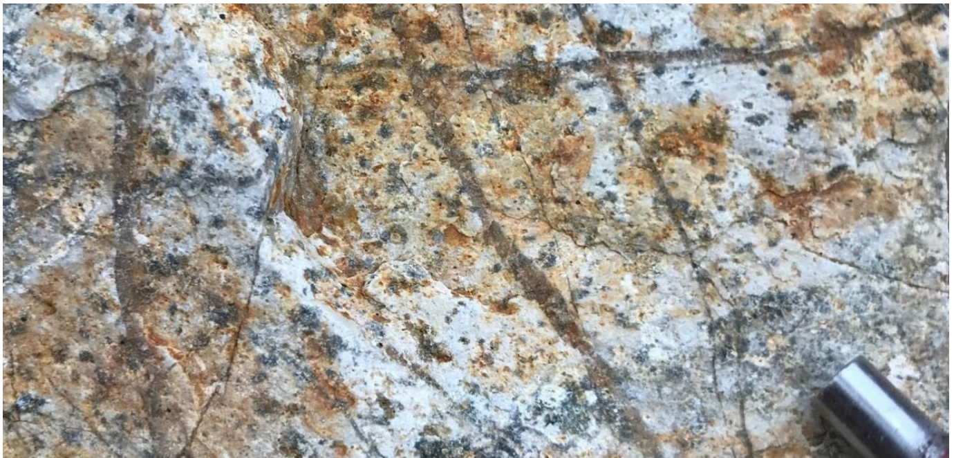
Plate 3. Translucent granular quartz veinlets associated with copper-gold mineralisation.
