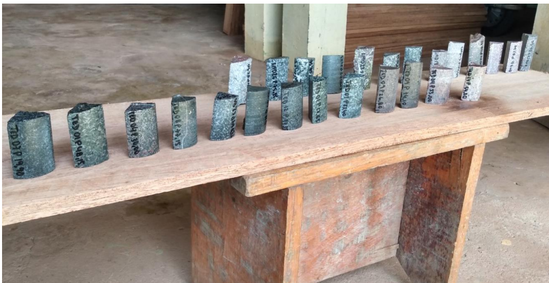
Figure 3: drill cores used in petrographic analysis
