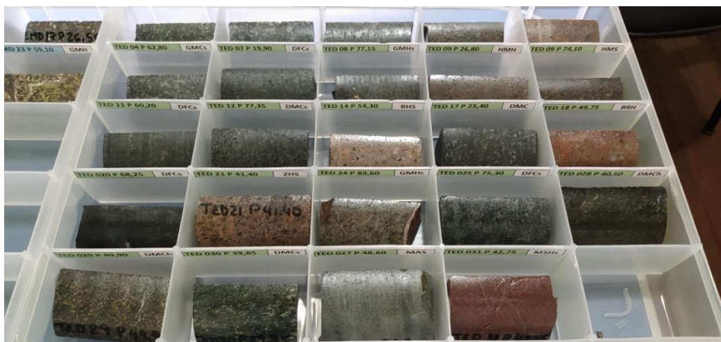
Figure 2: drill cores used in petrographic analysis
