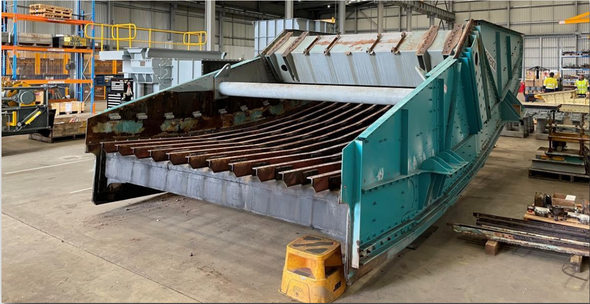
Figure 5: Schenck screen being refurbished at RCR
