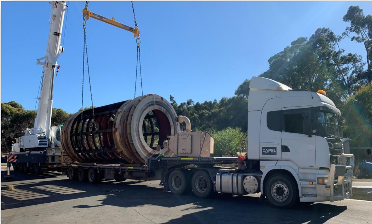
Figure 4: The trommel barrel is loaded for transport
