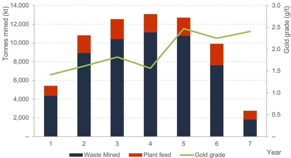
**Figure 1: Mining profile underpinning the 2022 FSU**
