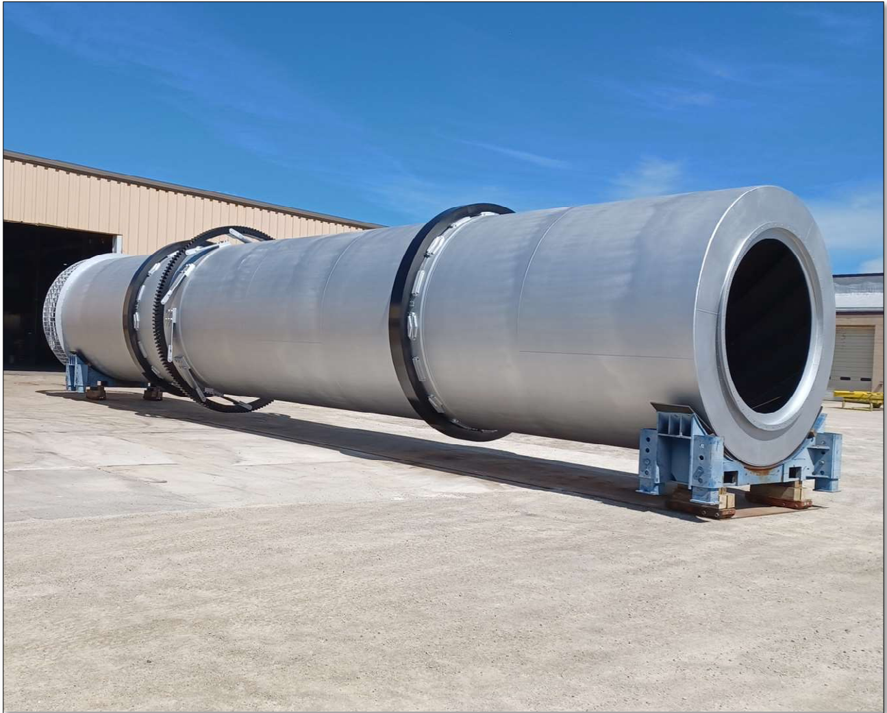
Figure 2 - Phosphate fertilizer plant dryer drum, ready to be shipped from FEECO headquarters USA.
