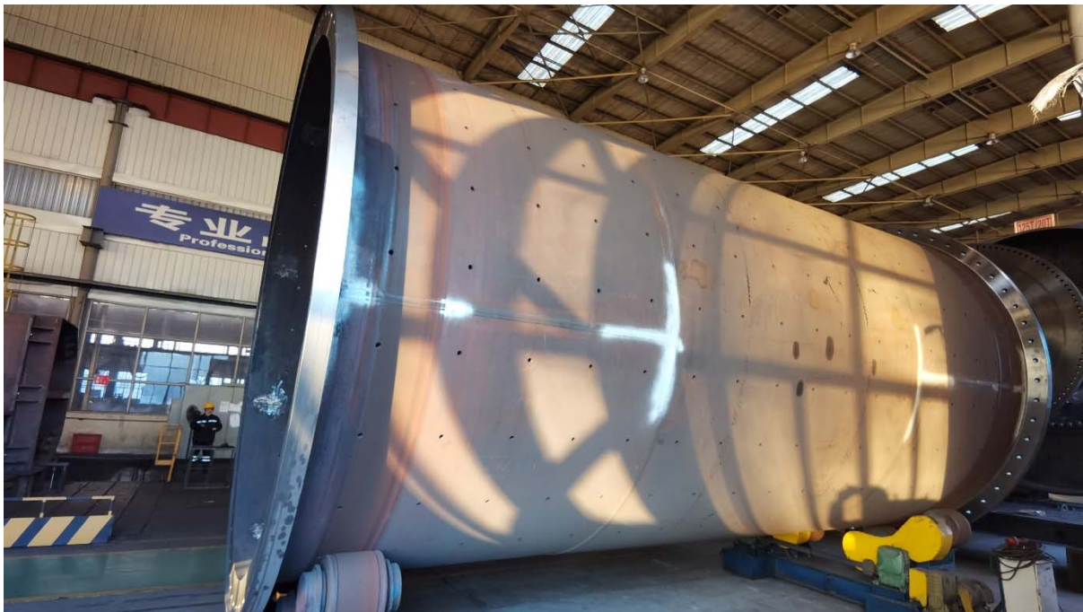
The Ball Mill Shell During Construction
