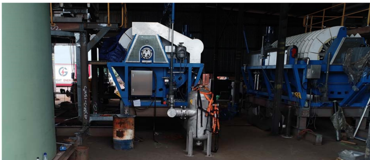
Two (2) Ceramic Disk Filters for de-watering final product
