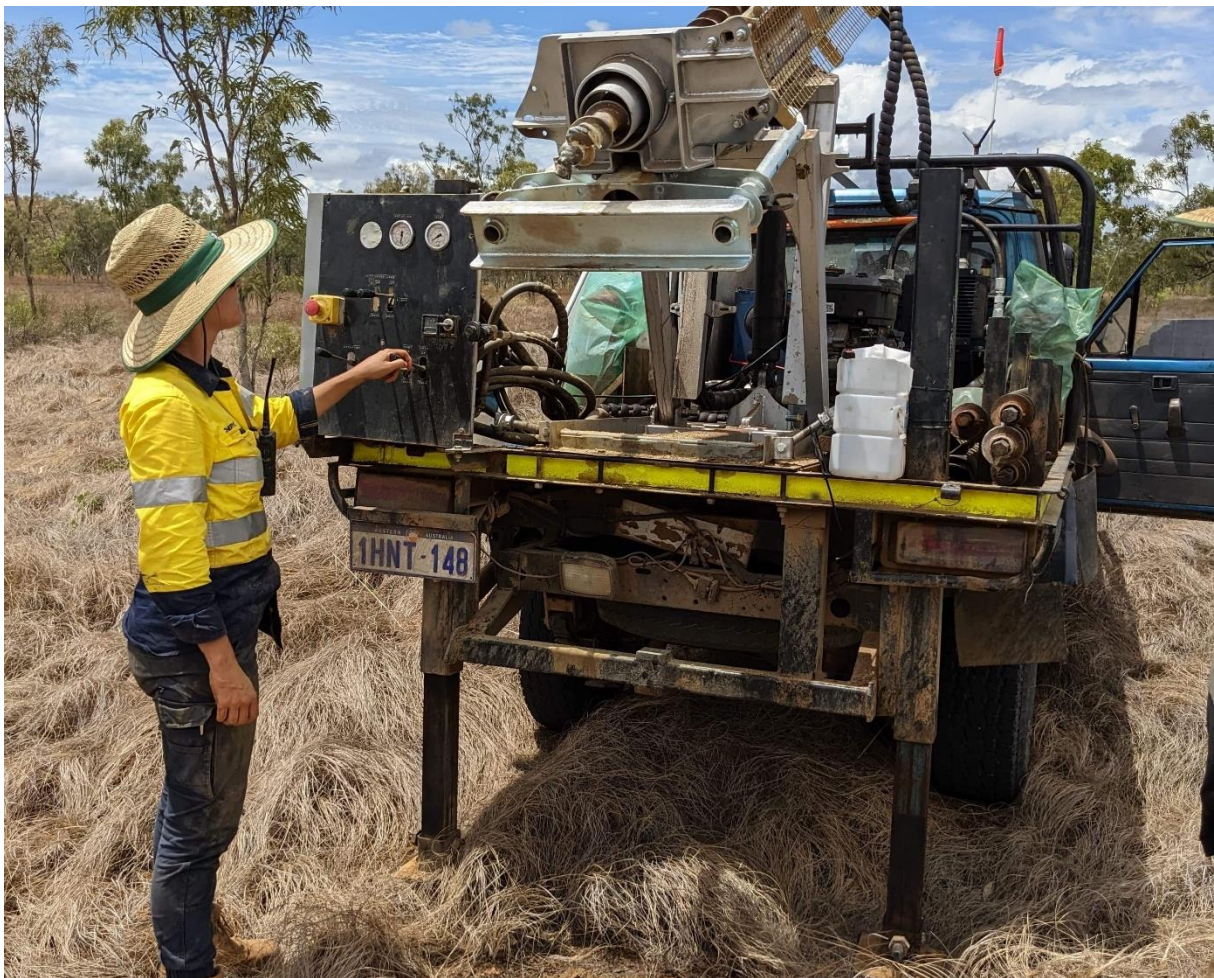
Figure 4: Cheryl Blessing from OzEx setting up the low-impact auger system over a sample location at Tarraji-Yampi.
