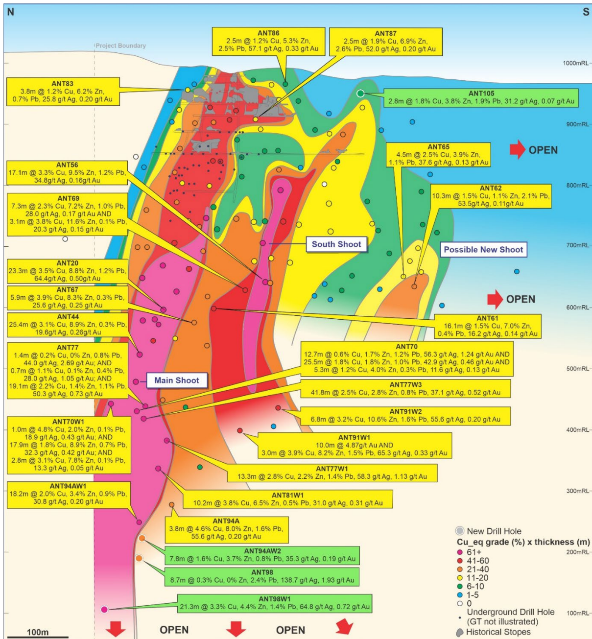
Figure 2. Long Section of grade x thickness for copper-equivalent results from the Antler Deposit showing historical underground workings, grade-thickness results for all surface drilling and select significant intersections in previous drilling (yellow text boxes for previously announced results and green text boxes for most recent results).
