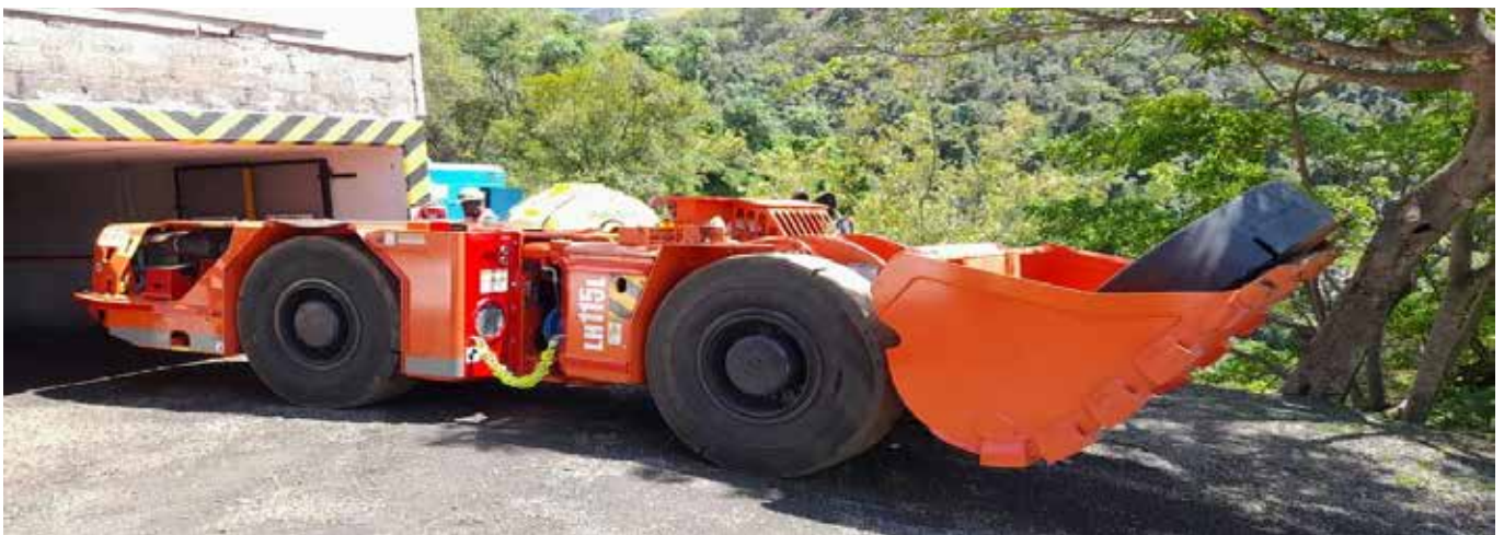
Figure 2: Low-Profile Loader entering Frankfort mine
