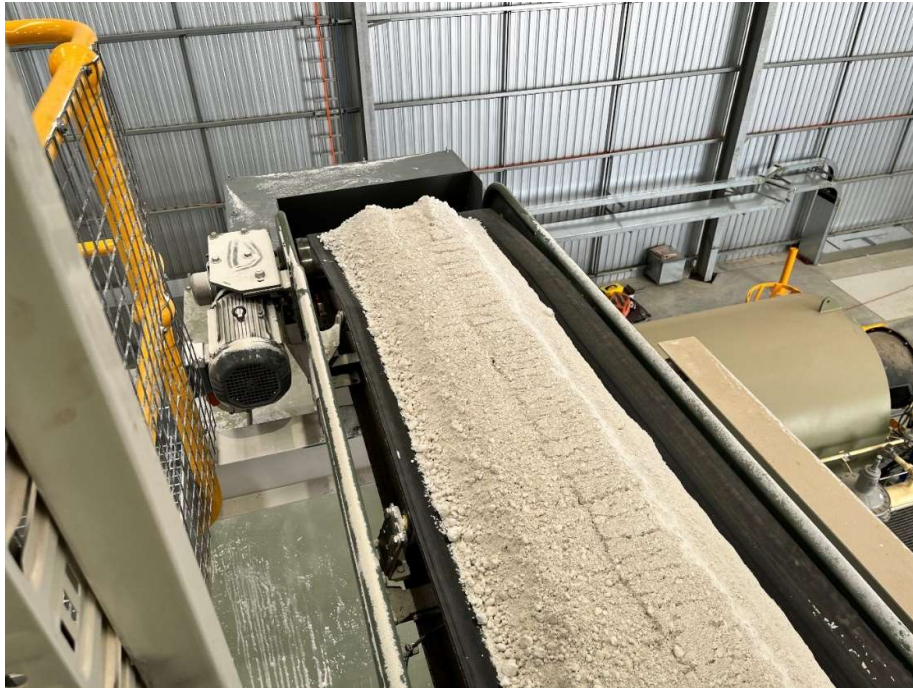
Figure 2. Conditioned ore being fed into rotary kiln
