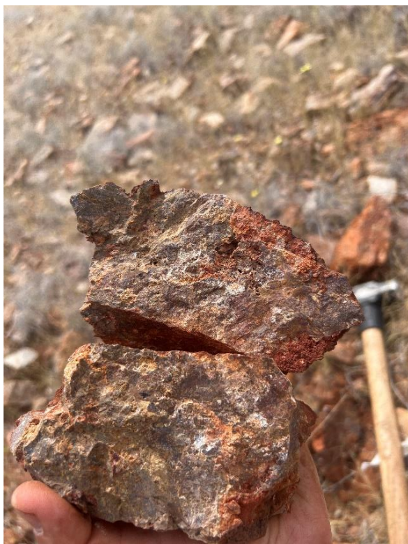
Figure 3: High grade monazite-rich samples MWGS1114 (left) and monazite rich sample MWGS0800 (right) which assayed 15.79% TREO with 2.41% \text{Nd}_2\text{O}_3 + \text{Pr}_6\text{O}_{11} and 13.30% TREO with 1.99% \text{Nd}_2\text{O}_3 + \text{Pr}_6\text{O}_{11} .
