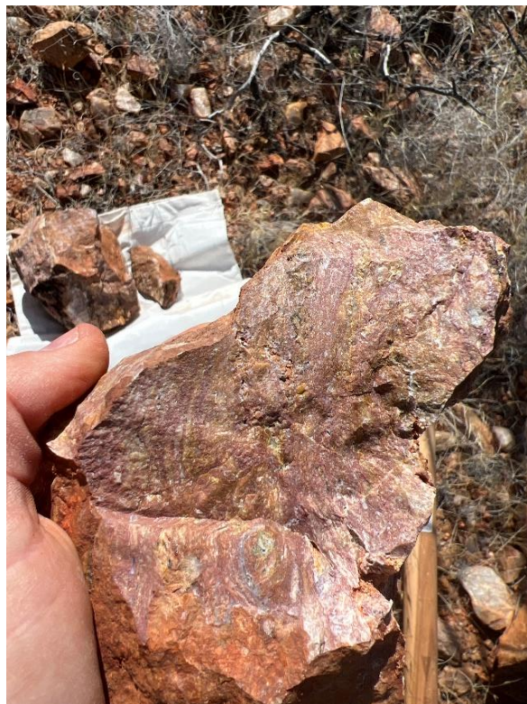
Figure 2: Massive monazite sample MWGS1108 (left) and MWGS0848 (right) which assayed 28.07% TREO with 4.63% \text{Nd}_2\text{O}_3 + \text{Pr}_6\text{O}_{11} and 23.81% TREO with 3.97% \text{Nd}_2\text{O}_3 + \text{Pr}_6\text{O}_{11} .
