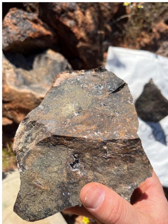
Figure 3: High grade monazite-rich samples MWGS1114 (left) and monazite rich sample MWGS0800 (right) which assayed 15.79% TREO with 2.41% \text{Nd}_2\text{O}_3 + \text{Pr}_6\text{O}_{11} and 13.30% TREO with 1.99% \text{Nd}_2\text{O}_3 + \text{Pr}_6\text{O}_{11} .
