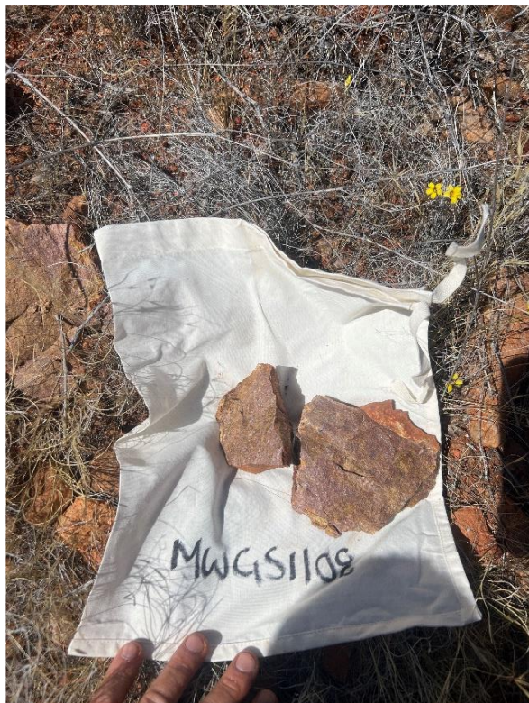
Figure 2: Massive monazite sample MWGS1108 (left) and MWGS0848 (right) which assayed 28.07% TREO with 4.63% \text{Nd}_2\text{O}_3 + \text{Pr}_6\text{O}_{11} and 23.81% TREO with 3.97% \text{Nd}_2\text{O}_3 + \text{Pr}_6\text{O}_{11} .
