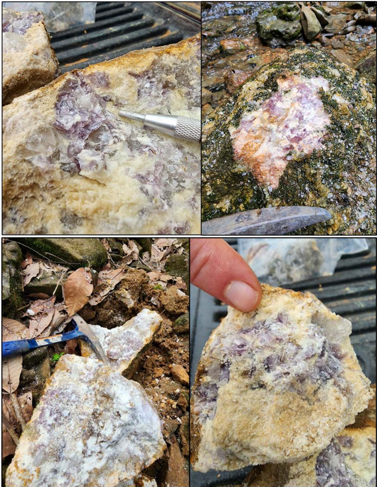
Photos: pegmatite with lepidolite (pink lithium bearing mica) discovered at Phang Nga (rock mass visually estimated to contain up to 40% lepidolite, top right photo)
