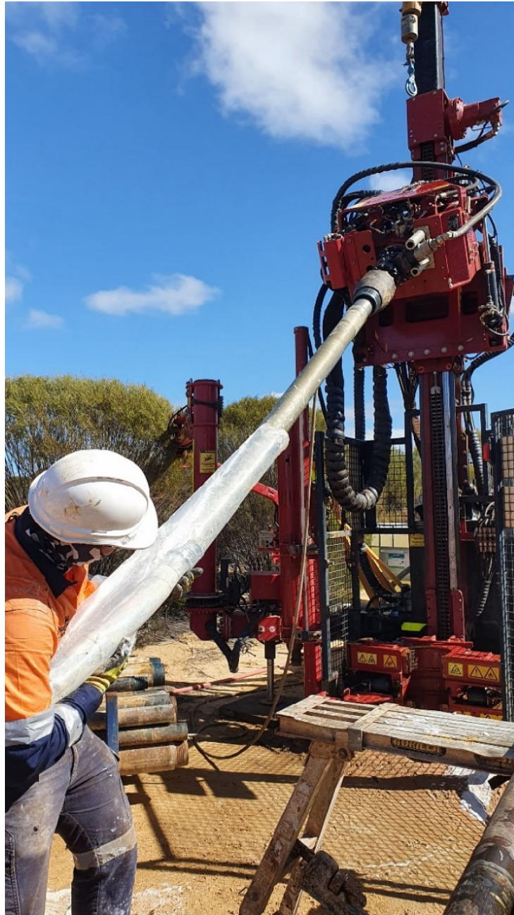
Figure 4: Resource Definition sonic core drilling at Tampu project
