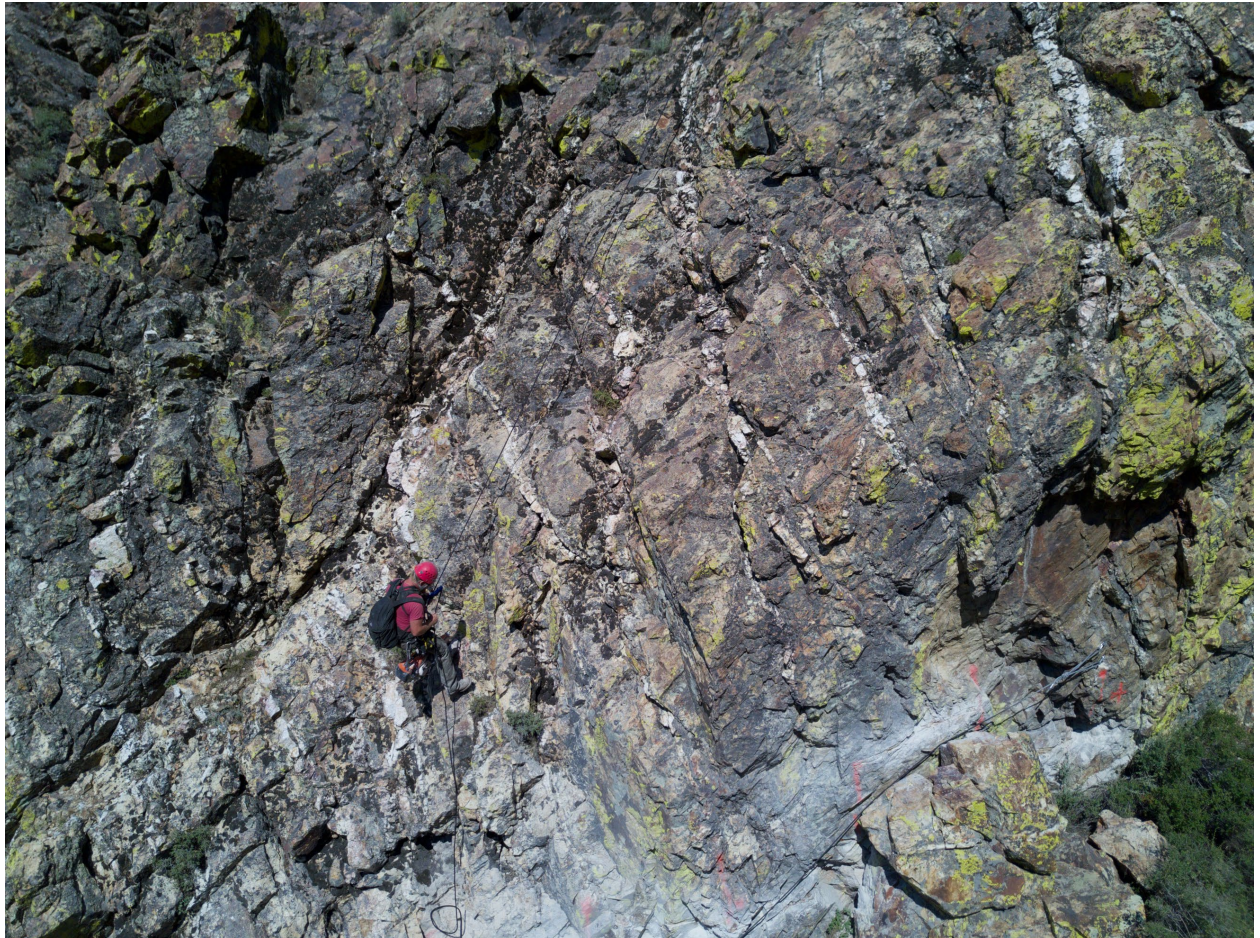
Figure 5. PolarX field crew saw-cutting channel sample across vein swarms host in rhyolite rocks at the Golden Staircase target, Humboldt Range, Nevada.
