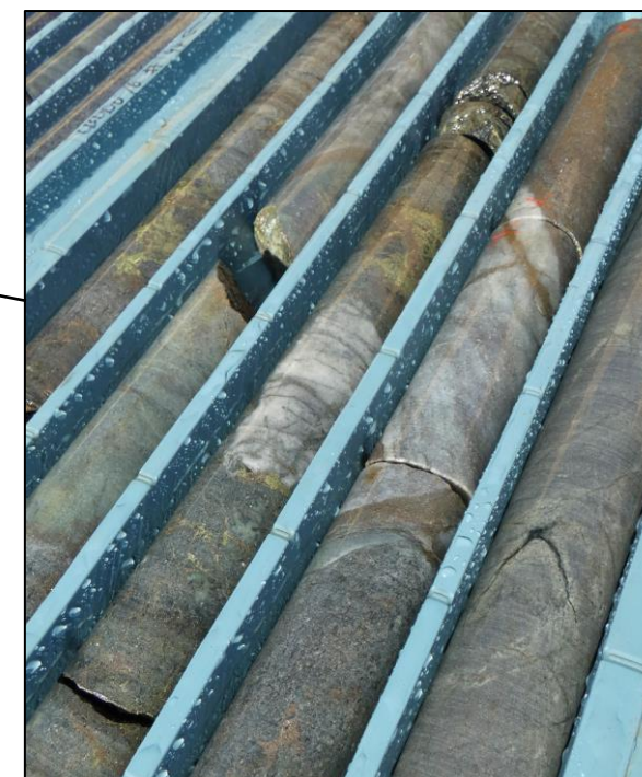
Broonhill core from CBDD076, 6.23m @ 0.6% Ni & 0.7% Cu
